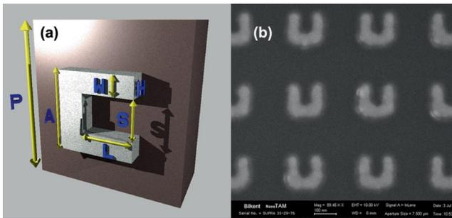
**Figure 1** (online colour at: www.pss-rapid.com) (a) Schematic and parameters of the unit cell. (b) Scanning electron microscopy image of the fabricated array.
