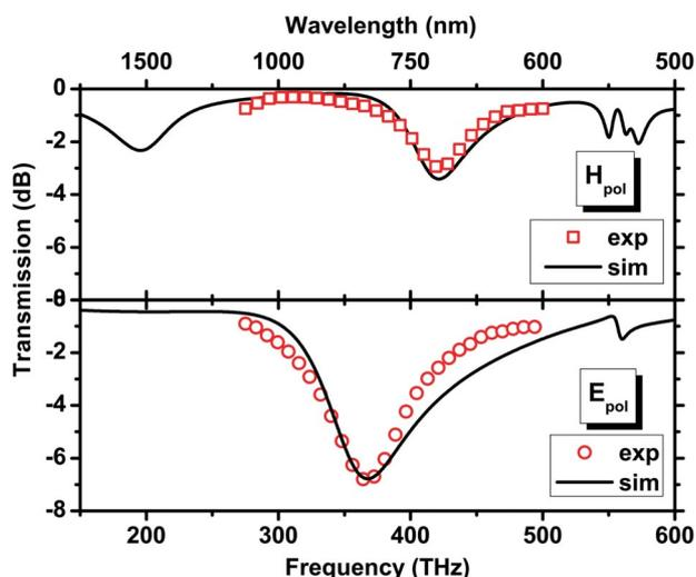
**Figure 2** (online colour at: www.pss-rapid.com) Simulated and measured transmission response of the sample SRR array.
