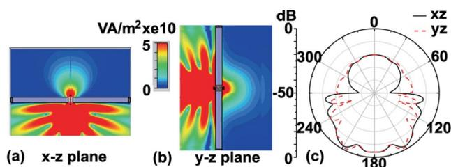
**Figure 4** (online colour at: [www.pss-rapid.com](http://www.pss-rapid.com)) Field distributions at 300 THz. Near field power distributions around the structure in the basis planes: (a)  $x-z$  plane, (b)  $y-z$  plane. (c) Far field patterns cut in the two planes.
