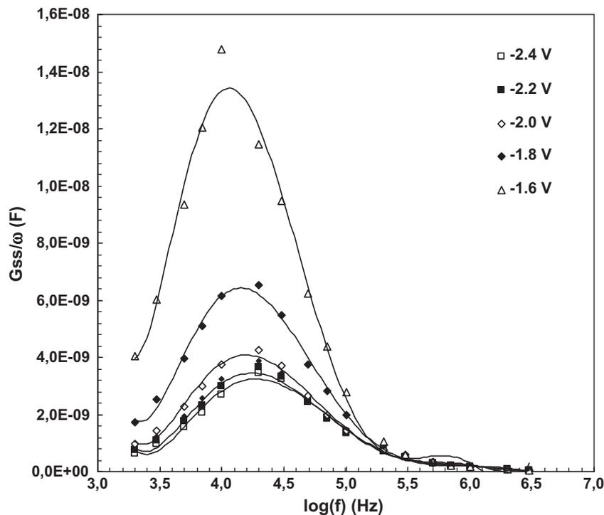
Fig. 9. The frequency dependence of  $G_{ss}$  characteristics obtained from the experimental forward bias capacitance and conductance measurements of (Ni/Au)/Al<sub>0.22</sub>Ga<sub>0.78</sub>N/AlN/GaN heterostructure at room temperature.
