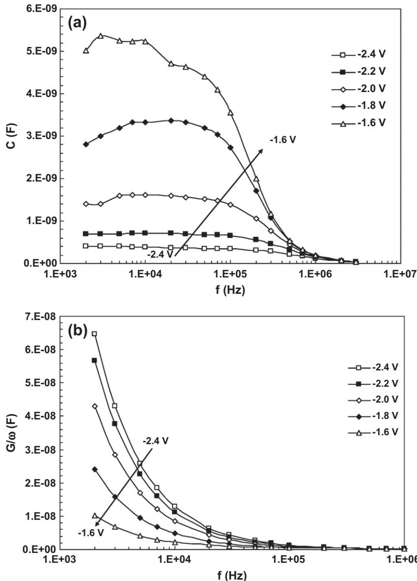
Fig. 8. The frequency dependence of: (a) the  $C(V_C)$ - $f$  and (b)  $G/\omega(V_C)$ - $f$  characteristics of the (Ni/Au)/Al<sub>0.22</sub>Ga<sub>0.78</sub>N/AlN/GaN heterostructure at room temperature.
