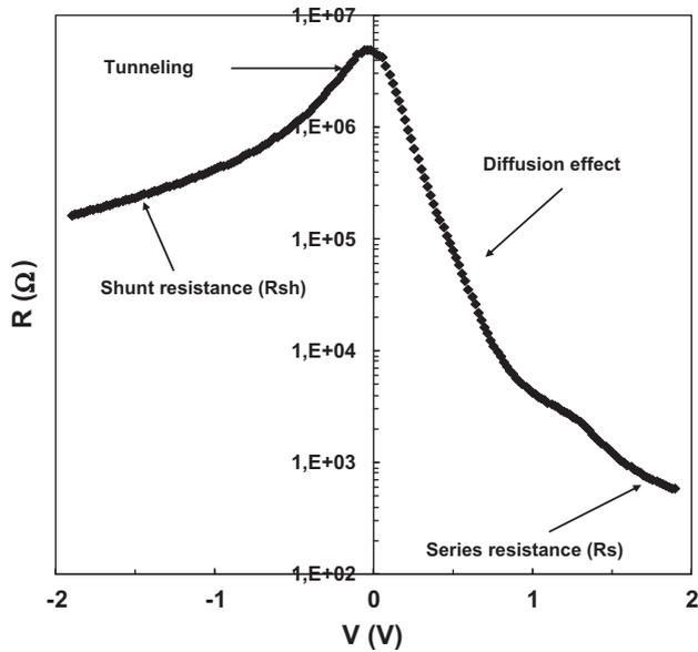
Fig. 3. The variation of  $R_s$  as a function of bias voltage for (Ni/Au)/Al<sub>0.22</sub>Ga<sub>0.78</sub>N/AlN/GaN heterostructure at room temperature.
