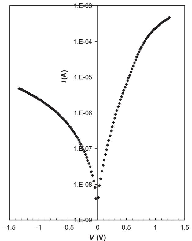
Fig. 2. Forward and reverse bias current-voltage ( $I-V$ ) characteristics of the Ni/Au)/Al<sub>0.22</sub>Ga<sub>0.78</sub>N/AlN/GaN heterostructure in semi-logarithmic scale at room temperature.
