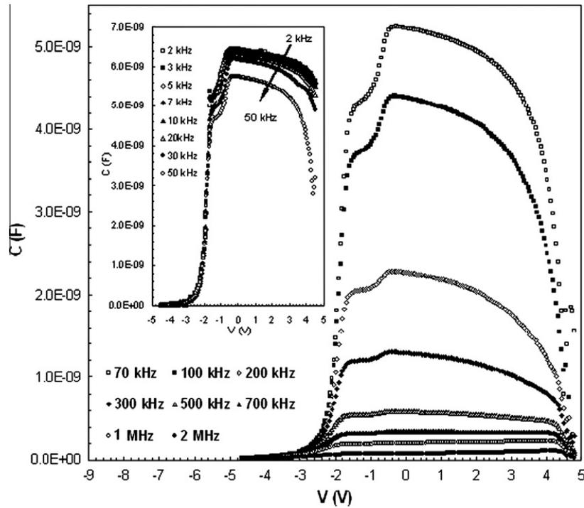
Fig. 5. The frequency dependent curves of the C–V characteristics of (Ni/Au)/Al<sub>0.22</sub>Ga<sub>0.78</sub>N/AlN/GaN heterostructure at room temperature.
