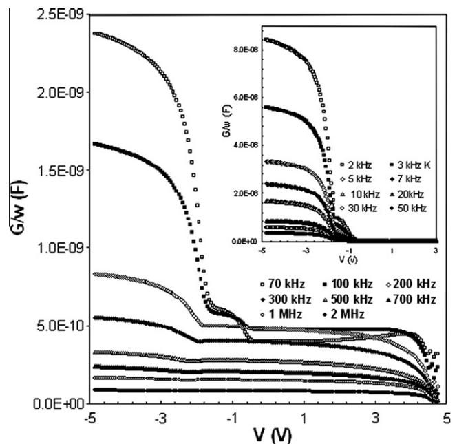
Fig. 6. The frequency dependent of  $G/\omega$ – $V$  characteristics for (Ni/Au)/Al<sub>0.22</sub>Ga<sub>0.78</sub>N/AlN/GaN heterostructure at room temperature.
