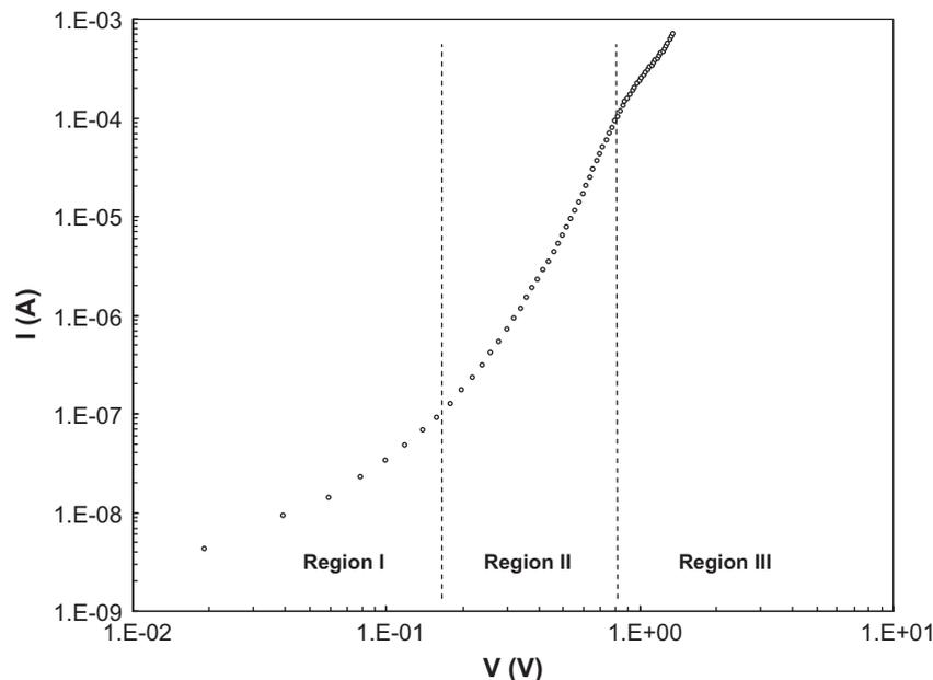
Fig. 4. The  $\ln(I)$  vs.  $\ln(V)$  characteristics of the (Ni/Au)/Al<sub>0.22</sub>Ga<sub>0.78</sub>N/AlN/GaN heterostructure at room temperature.
