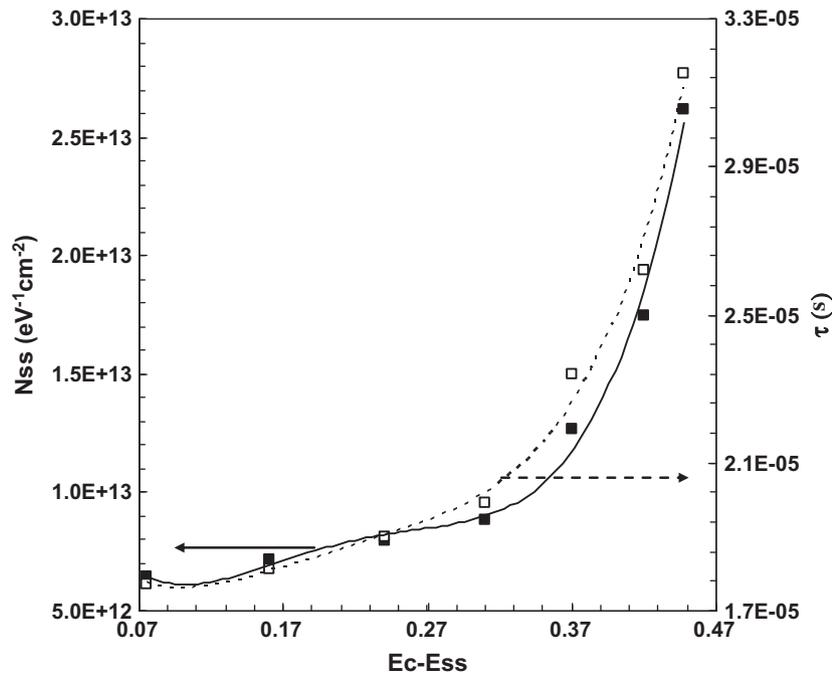
Fig. 11. The energy distribution of interface states and their time constant obtained from conductance method for  $(\text{Ni}/\text{Au})/\text{Al}_{0.22}\text{Ga}_{0.78}\text{N}/\text{AlN}/\text{GaN}$  heterostructures at room temperature.
