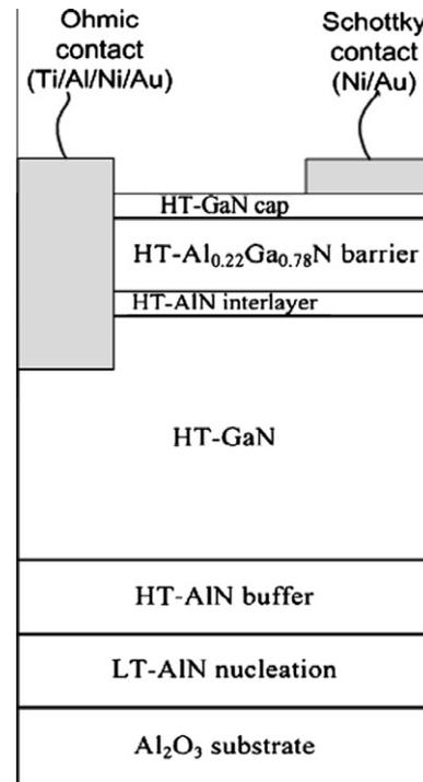
Fig. 1. Schematic diagram of the (Ni/Au)/Al<sub>0.22</sub>Ga<sub>0.78</sub>N/AlN/GaN heterostructures and a view of ohmic and Schottky contacts on the structures.
