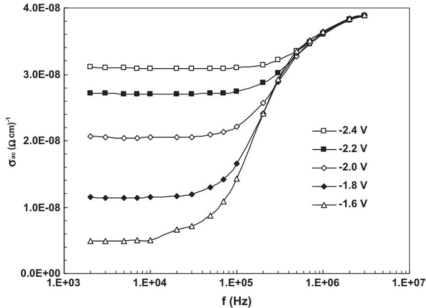
Fig. 12. Frequency dependence of ac electric conductivity ( $\sigma_{ac}$ ) for various applied voltage of (Ni/Au)/Al<sub>0.22</sub>Ga<sub>0.78</sub>N/AlN/GaN heterostructures at room temperature.
