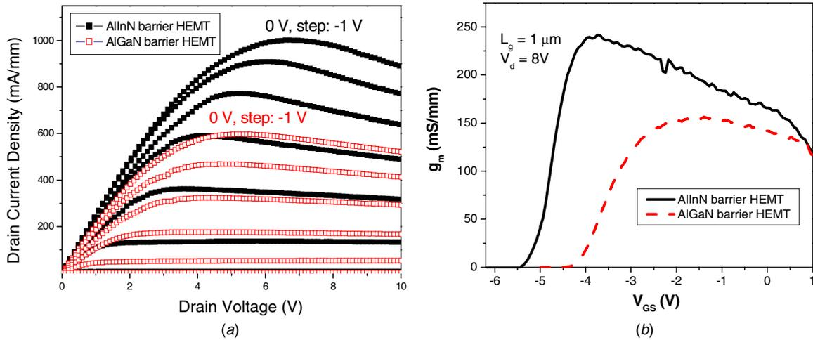
**Figure 4.** DC—IV output characteristics (a) and extrinsic transconductance (b) of the conventional  $\text{Al}_{0.3}\text{Ga}_{0.7}\text{N}$  barrier HEMT and  $\text{Al}_{0.83}\text{In}_{0.17}\text{N}$  barrier HEMT.
