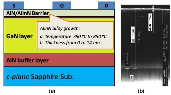
**Figure 1.** Schematic cross-sectional view of the AlInN barrier HEMT structure (a) and a corresponding SEM image (b).
