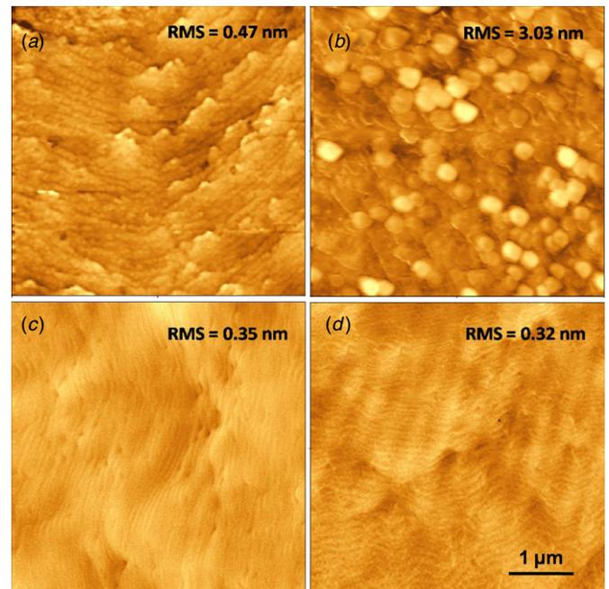
**Figure 6.** AFM images of HEMT epitaxial structures after thermal annealing: (a) and (b)  $\text{Al}_{0.83}\text{In}_{0.17}\text{N}$  barrier HEMT annealed at  $700$  and  $800 \text{ }^\circ\text{C}$ , respectively; (c) and (d)  $\text{Al}_{0.3}\text{Ga}_{0.7}\text{N}$  barrier HEMT annealed at  $700$  and  $800 \text{ }^\circ\text{C}$ , respectively.
