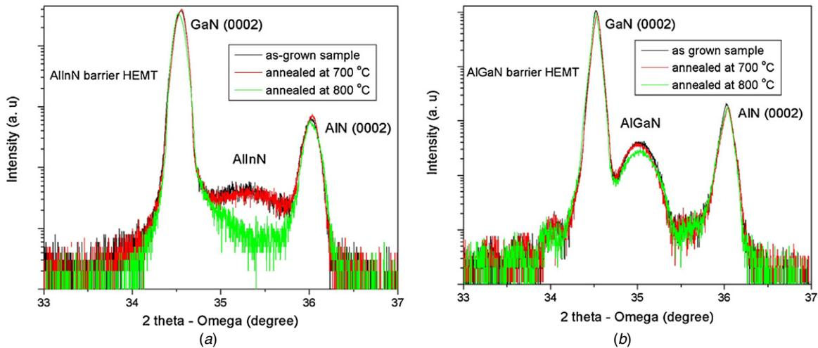
**Figure 5.** XRD  $2\theta$ - $\omega$  scans of the (0002) reflection for the HEMT structures thermally annealed at various temperatures for 30 min. Two kinds of the HEMT structures are shown with (a)  $\text{Al}_{0.83}\text{In}_{0.17}\text{N}$  barrier and (b)  $\text{Al}_{0.3}\text{Ga}_{0.7}\text{N}$  barrier.
