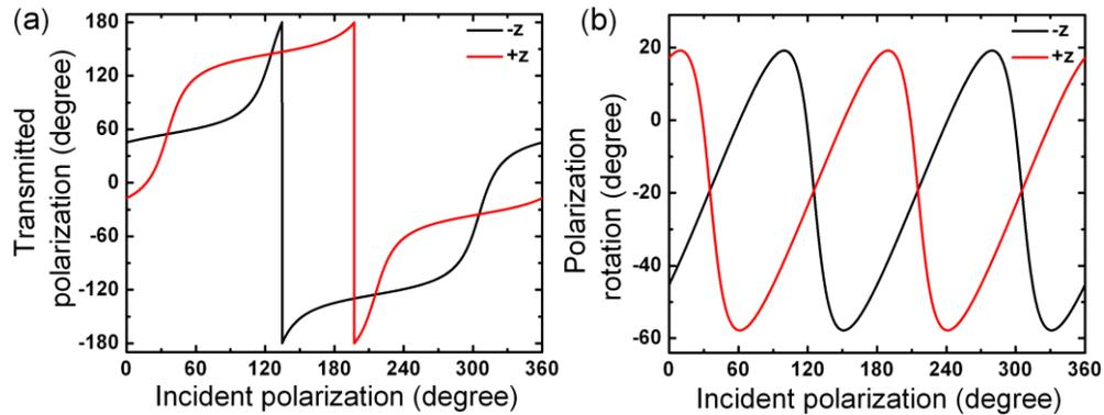
Fig. 6. (a) Polarization angles of the transmitted linearly polarized waves with respect to the polarization angle of the incident wave, at 6.2 GHz, for the  $-z$  and  $+z$  propagating waves (b) Introduced polarization rotation to the  $-z$  and  $+z$  propagating waves with respect to the incident polarization angle, at 6.2 GHz.
