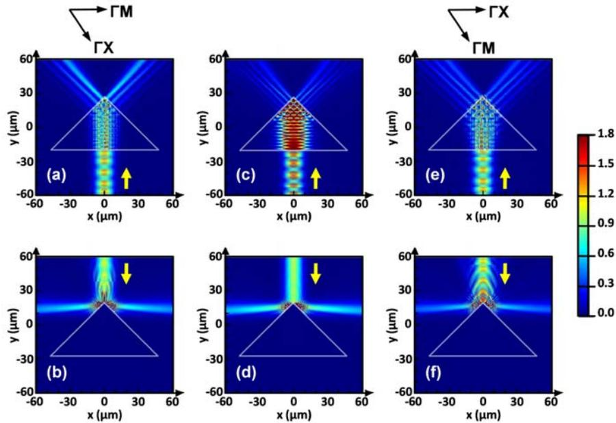
Fig. 3. Electric field distribution at 179 THz ( $ka = 3.75$ ): for PhC prism at (a) forward-case (here -  $\Gamma M$  interface) illumination and (b) backward-case (wedge) illumination; for non-magnetic ULIM prism with  $n = 0.22$  at (c) forward-case (here - longer-side) illumination and (d) backward-case (wedge) illumination; for PhC prism at (e) forward-case ( $\Gamma X$  - interface) illumination and backward-case (wedge) illumination; yellow arrows show directions of beam incidence.
