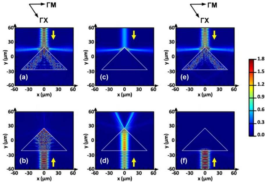
Fig. 5. Electric field distribution for (a) backward-case (here - wedge) illumination and (b) forward-case (here -  $\Gamma M$  interface) illumination for PhC prism at 207 THz ( $ka = 4.335$ ); (c) backward-case (here - wedge) illumination and (d) forward-case (here - normal, longer-side) illumination for non-magnetic ULIM prism with  $n = 0.59$  at 207 THz; (e) and (f) same as (a) and (b) but at 209 THz ( $ka = 4.4$ ); yellow arrows show directions of beam incidence.
